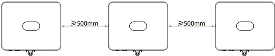
Fig. 4.5 Installation Dimension of Side-by-side Inverters
